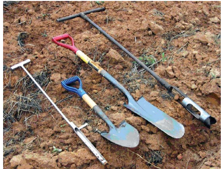
Figure 1. Examples of soil sampling options. From left, soil probe, spade, sharpshooter and soil auger.
