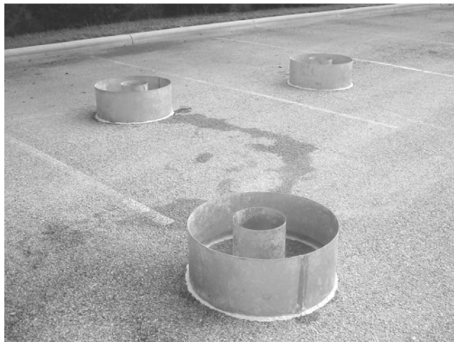
Fig. 2. Double-ring infiltrometer test
